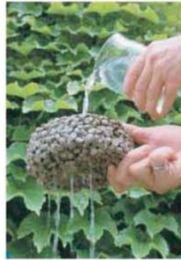
Pervious concrete pavement
